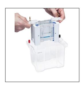
NOTE: It is best to turn the cams in opposite directions to each other. Do not overturn as this will cause the glass plates to push upwards and the assembly will be more likely to leak. The unit is now ready for gel preparation and pouring.
